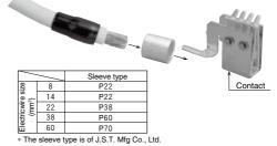
(4) Cover the crimped sleeve with the insulation cap.
