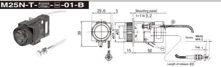
Illuminated type pushbutton with 1C contact and 1 release
