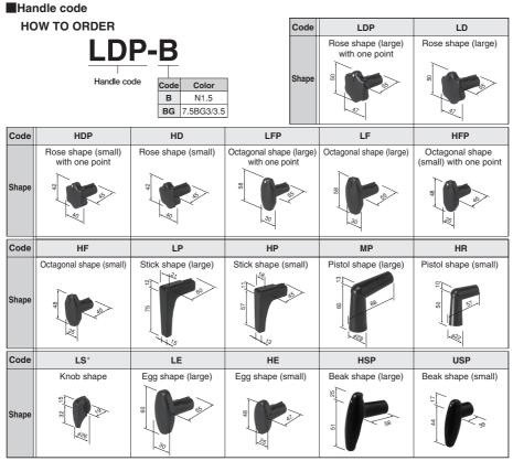
\* The shaft for the LS handle is 13 mm shorter than the standard shaft. Therefore, other types of handles cannot be replaced with the LS handle (knob shape).
