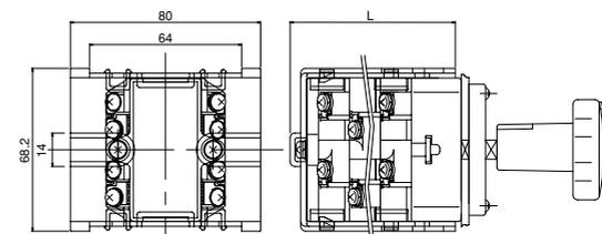
Note: This cover cannot be used for a rear terminal type and a dual-body type.
