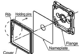
Rib within the cover can be attach any directions (up or down, left or right) to the flange.
